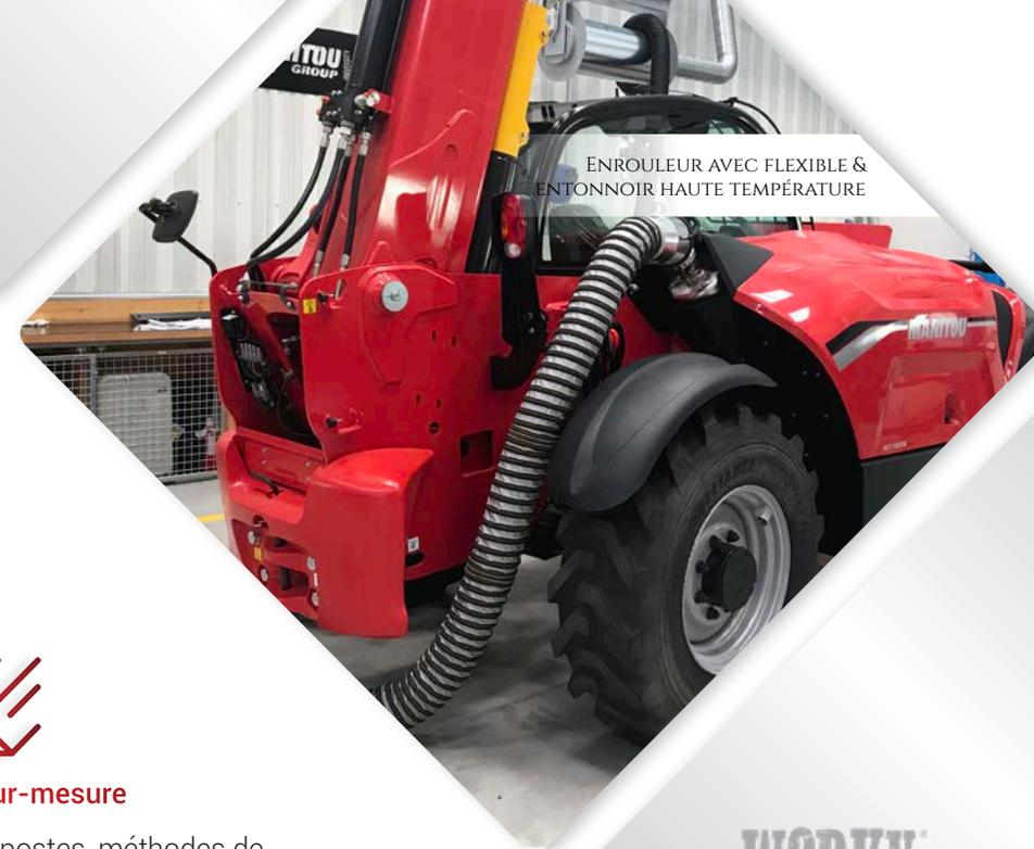
ENROULEUR AVEC FLEXIBLE & ENTONNOIR HAUTE TEMPÉRATURE
